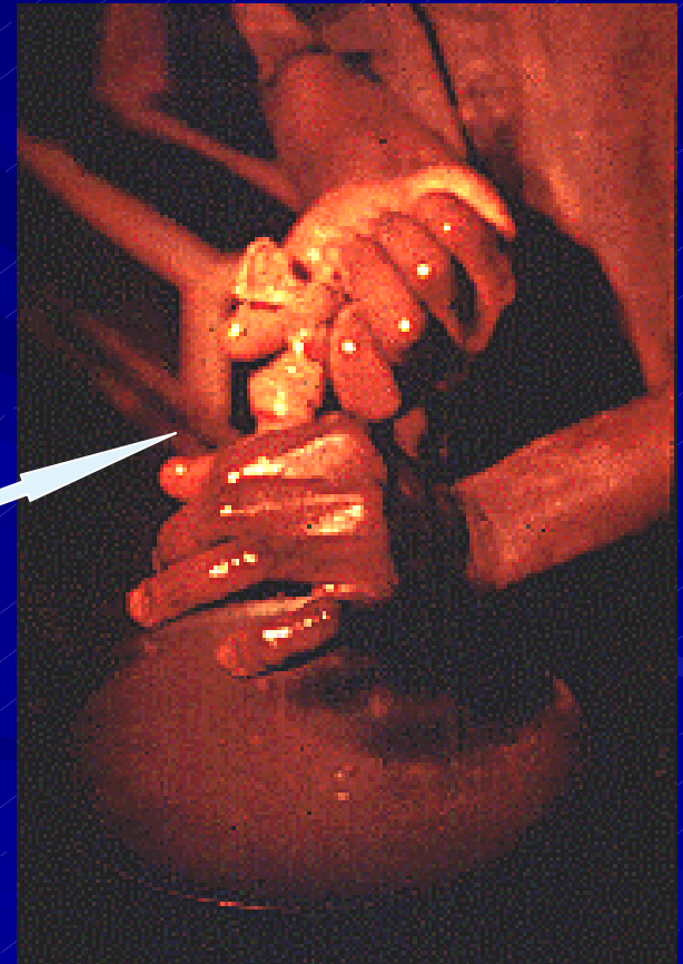
Mercury amalgamation in a batea
