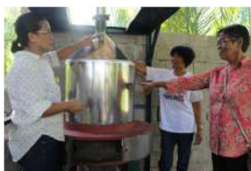
Lead Investigator Dr. Shirley Agrupis (left) examines the bioethanol facility installed at the Nipa Wine Making Cooperative in Pamplona, Cagayan. Photo by RTI International.
